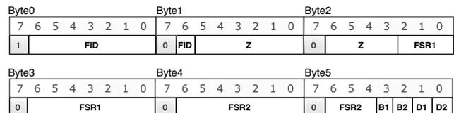
Figure 4: Overview of the SmartFiducial Serial Protocol
