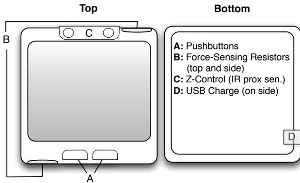
Figure 2: SmartFiducial Hardware Design Layout
